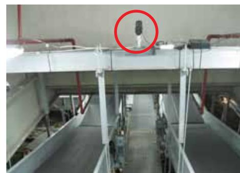
Due to the wide angle lens one FLIR A310 thermal imaging camera can cover two conveyor belts.
